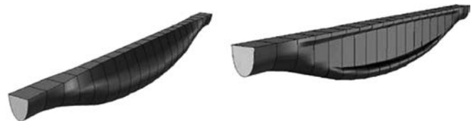
Figure 7. Optimized beam shapes (Ibell 2009)
