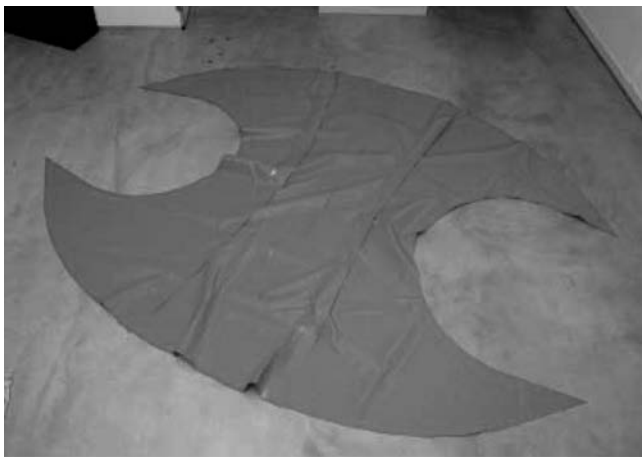
Figure 16. Fabric formwork after assembly of the fabric pieces
