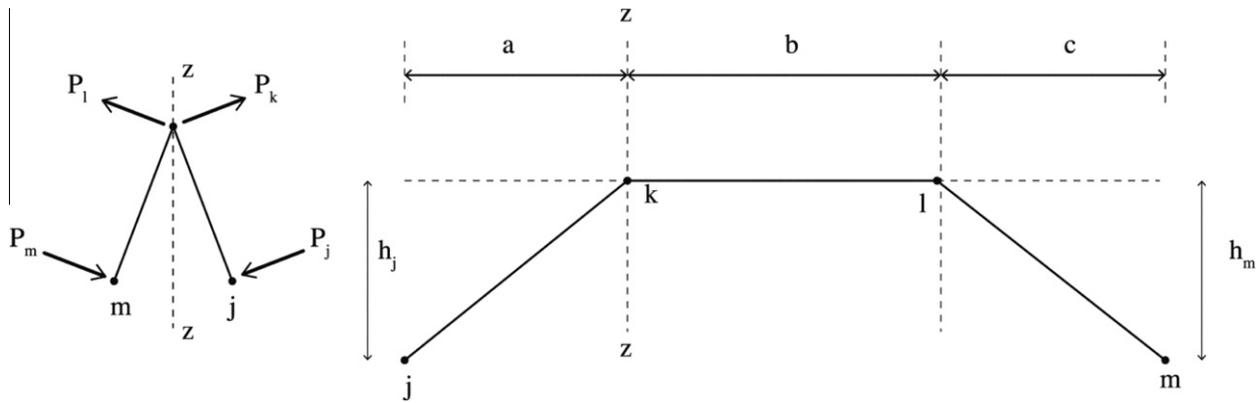
**Fig. 5.** Static equilibrium of the three link unit and side view with dimensions (note that the plane containing axis  $z-z$  and link  $kl$  bisects the planes  $jkl$  and  $klm$ ).
