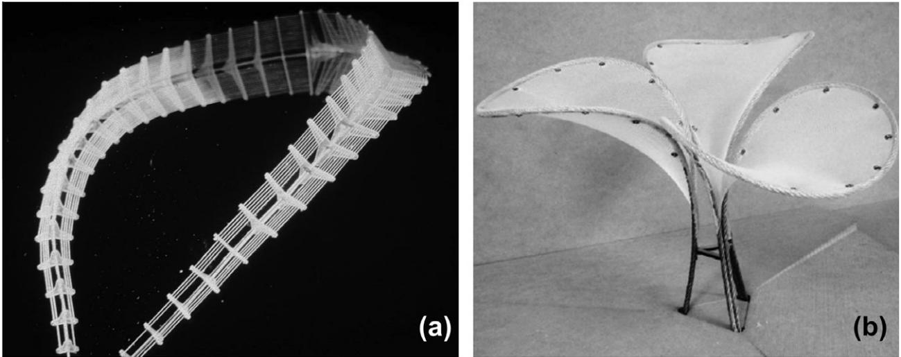
**Fig. 1.** (a) Crane model, a central flexible curved element is shaped by three sets of longitudinal cables (photo courtesy ILEK, Institut für Leichtbau Entwerfen und Konstruieren) and (b) a twisted and bent element equilibrates with a pre-stressed membrane to form a sun shading structure. (Princeton University student project photo courtesy S Bagrianski, A Heid and M Krupka.)
