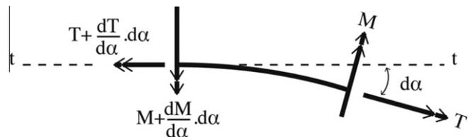
Fig. 3. Free body diagram for a small element of a curved member.
