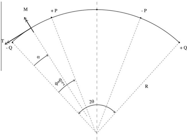
Fig. 7. A circular arc beam with radius  $R$  with equal and opposite transverse loads  $P$  at the quarter points.
