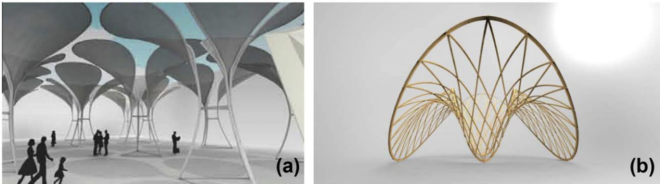
**Fig. 8.** (a) Solar shade that derives its shape from a doubly curved membrane pre-stressed against a three-dimensional curved flexible element (PU student project image courtesy S. Bagrianski, A. Heid, M. Krupka). (b) The initial shape of a strained grid shell accounts for straining due to bending and torsion. (SG gridshell image courtesy A. Kudless, M. Cabrinha and D. Shook).
