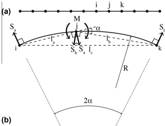
Fig. 2. (a) Consecutive nodes along an initially straight tubular beam traverse; (b) two adjacent deformed segments, a and b, viewed normal to the plane  $ijk$ .
