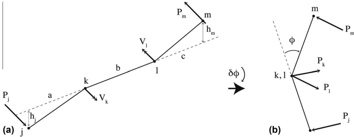
Fig. 6. Forces acting on a curved element with inflected sections ((a) perspective and (b) view parallel with  $kl$ ).
