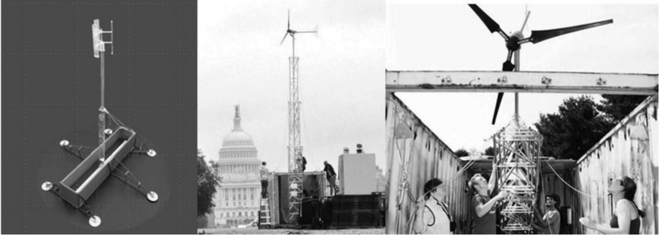
Fig. 1. (Left) Physical model; (middle and right) full-scale prototype for “Power in a Box,” a telescoping mast with a wind turbine mounted on a transportable standard steel shipping container (“Power in a Box,” Princeton University; middle photo courtesy of Catherine Peters; right photo courtesy of Frank Wojciechowski).
