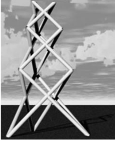
Fig. 2. Conceptual rendering of the three-dimensional tetrahedral pantograph mast.
